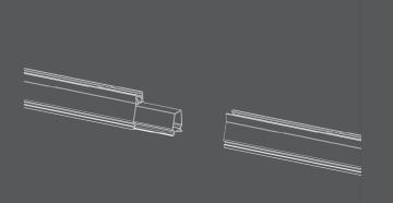
4. The internal rail joiner ensures earth continuity between rails without obstructing component attachment. It seamlessly slides inside the Nova rail, allowing for a smooth and uninterrupted join.
