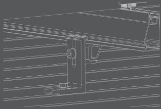
2.The L Feet allows for a considerable range of height adjustability paired with an embedded EPDM rubber for superior water sealing.
