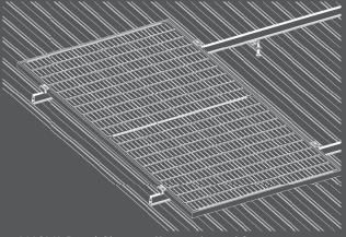
6.NOVA Panel Clamps offer a universal fit, accommodating panel thickness ranging from 30mm to 40mm.
