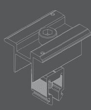
5.The NOVA panel clamps incorporates a user-friendly Clip-in design and integrated earthing pins, eliminating the requirement for an additional grounding plate.
