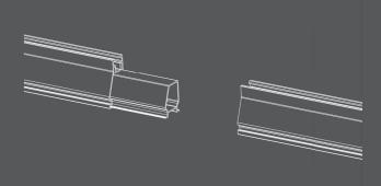
4. The internal rail joiner ensures earth continuity between rails without obstructing component attachment. It seamlessly slides inside the Nova rail, allowing for a smooth and uninterrupted join.
