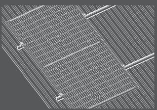
6.NOVA Panel Clamps offer a universal fit, accommodating panel thickness ranging from 30mm
