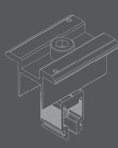
5.The NOVA panel clamps incorporates a user-friendly Clip-in design and integrated earthing pins, eliminating the requirement for an additional grounding plate.
