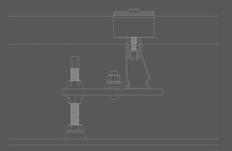
2. Height adjustablity for roofing clearance.
