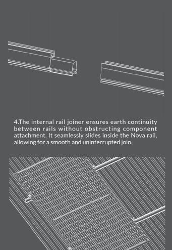
6.NOVA Panel Clamps offer a universal fit, accommodating panel thickness ranging from 30mm to 40mm.
