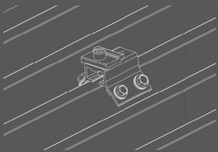
2. Includes EPDM rubber padding for watertight sealing.
