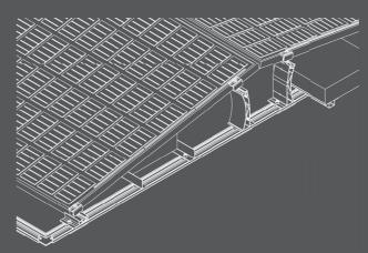
5.Strategically engineered for optimal strength and cost-effectiveness, our front and rear legs utilize triangular mechanics to maximize structural integrity without compromising value.
