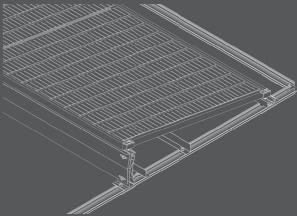
2.Enhance stability with our versatile ballast trays, designed for compatibility with various concrete types. The unique structure ensures increased stability across the entire array.
