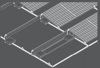
3. The EPDM Base offers enhanced friction with the roof, providing cushioning and protection. Its raised design allows for proper water drainage, effectively preventing corrosion.
