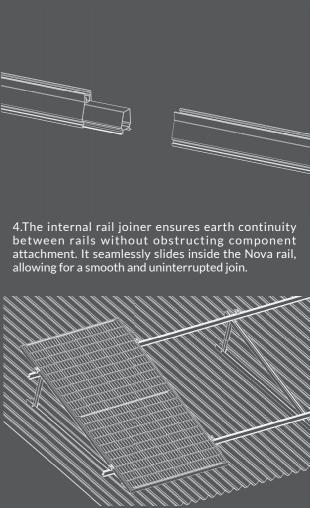
6.NOVA Panel Clamps offer a universal fit, accommodating panel thickness ranging from 30mm to 40mm.
