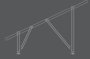
4.Strategically engineered for optimal strength and cost-effectiveness, The W shape structure utilizes triangular mechanics to maximize structural integrity without compromising value.
