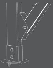
5. The base is securely fixed to the ground using anchor screws, while the column is locked in place with carbon steel bolts, ensuring stability and preventing any loosening or displacement.
