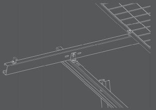
3. Rails are easily installed to the upright structural support using our rail clamp.
