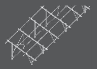
1.Manufactured from Zinc-Aluminum-Magnesium Coated Steel, our products offer superior corrosion resistance, surpassing that of galvanized steel.
