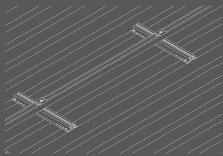
2. Direct attachment onto the metal roof.
