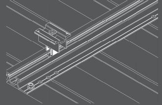
4.Panel clamps feature a clip in mechanism for easy installation onto the MINI rail.
