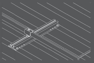
3.Each MINI Rail includes a EPDM rubber base pad that cushions the system against the mounting surface and provides waterproofing.
