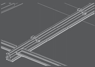
2. The NOVA ZERO Railing System features integrated water drainage channels, ensuring effective water management and preventing pooling or accumulation.
