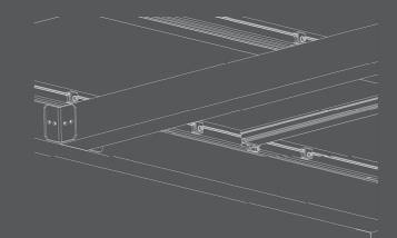
3.The strategically designed purlins feature prethreaded holes, providing convenient railing installation.
