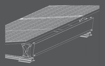
4. The front and rear legs feature prethreaded holes for wind deflector installation, enhancing array stability and ensuring the safety of the PV system.
