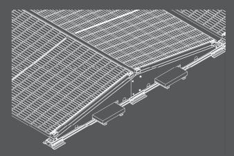
5. The short-side wind deflector conveniently accommodates cable and ballast outlets, greatly simplifying cable and ballast installation management.
