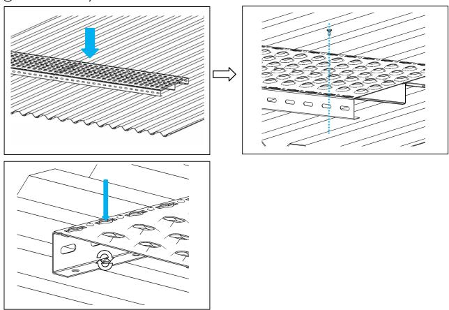
Tighten the self-tapping screws
