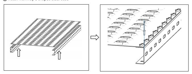
Connect the walkway pedal with the C-shaped steel base by rivets
