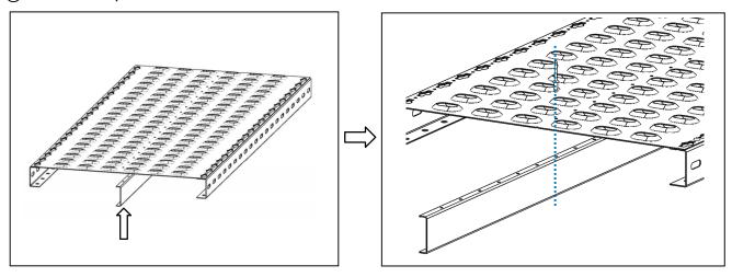
Walkway board fixed the center beam with Rivets (suggestion: the center beam extend beyond the walkway board 300mm)
