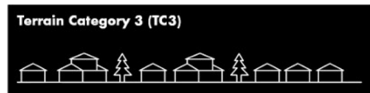
Terrain Category 3 (TC3) Site surrounded by trees or buildings 3m to 5m high (typical suburban site).
