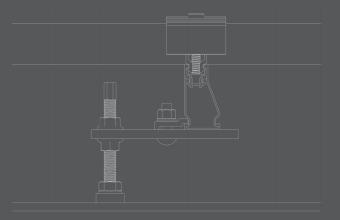
2. Height adjustablity for roofing clearance.
