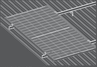
6.NOVA Panel Clamps offer a universal fit, accommodating panel thickness ranging from 30mm to 40mm.
