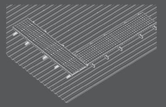
1. Manufactured from Zinc-Aluminum-Magnesium Coated Steel, our products offer superior corrosion resistance, surpassing that of galvanized steel.
